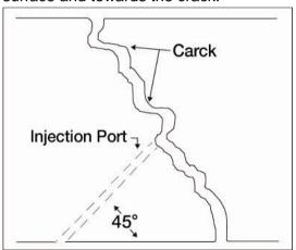
The depth of the drill hole intersecting the crack should be somewhere close to the middle of structure, if possible. Holes deeper than 30cm are usually not required even if the concrete being repaired is more than 100cm thick.
